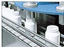
Indexing disc with insert tube. Film cut, folded, inserted into tube, transferred and inserted into bottle by intermittent index drive.
