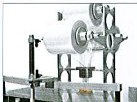
Roll PE film supply reel. The number of rolls determined by container ullage.
