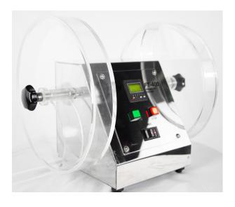
The Key Friability Tester (FT-400) is a mechanical apparatus used to determine or test tablets for resistivity to breakage. The resistivity to breakage can be measured by using the "ROCHE" test which subjects the tablets to mechanical shock in order to establish a friability factor based on the loss in tablet weight due to breakage caused by induced mechanical stress. The FT-400 conforms completely to the test parameters as established by "ROCHE" as outlined in our technical section.
