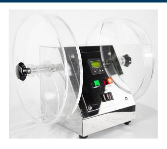
The Key Friability Tester (FT-400) is a mechanical apparatus used to determine or test tablets for resistivity to breakage. The resistivity to breakage can be measured by using the "ROCHE" test which subjects the tablets to mechanical shock in order to establish a friability factor based on the loss in tablet weight due to breakage caused by induced mechanical stress. The FT-400 conforms completely to the test parameters as established by "ROCHE" as outlined in our technical section.
