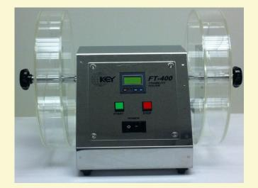
The Key Friability Tester (FT-400) is a mechanical apparatus used to determine or test tablets for resistivity to breakage. The resistivity to breakage can be measured by using the "ROCHE" test which subjects the tablets to mechanical shock in order to establish a friability factor based on the loss in tablet weight due to breakage caused by induced mechanical stress. The FT-400 conforms completely to the test parameters as established by "ROCHE" as outlined in our technical section.
