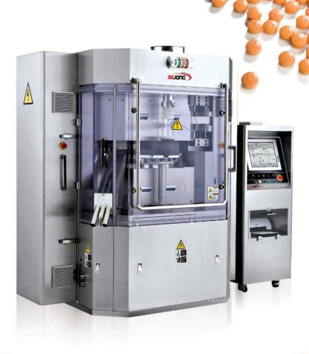
One of the key features of MRC-D series lies in the fact that it can produce double-layer tablets and in case of the production of single-layer tablets, it is possible to increase productivity two-fold by applying a double-sided discharge system.
