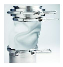
The CORA COMPENSATOR is a flexible sleeve that connects two pieces of machinery when rigid connections cannot be used due to vibration or off-axis. It can also be used in light overpressure/depression. The CORA COMPENSATOR is connected through a clamp band that can be opened easily when you need to sterilize the sleeve. It is also available with copper wire to ensure electrical conductivity.
