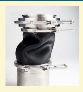
The CORA COMPENSATOR is a flexible sleeve that connects two pieces of machinery when rigid connections cannot be used due to vibration or off-axis. It can also be used in light overpressure/depression. The CORA COMPENSATOR is connected through a clamp band that can be opened easily when you need to sterilize the sleeve. It is also available with copper wire to ensure electrical conductivity.
