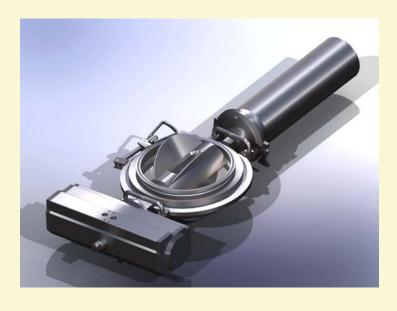
The CORA RV-SR Rotary Dosing Valve is a solution designed for accurate dosing and consists of two concentric rotors of different volume individually operated, which determine product flow and dosing. The main rotor ensures continuous product flow while the secondary rotor ensures accurate dosing. The CORA RV-SR is typically used in feeding packaging machines, drum & bag filling systems, and for dispensing
