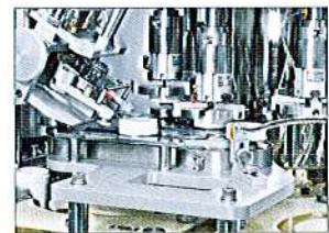
Cap feeder and pick & place mechanism
