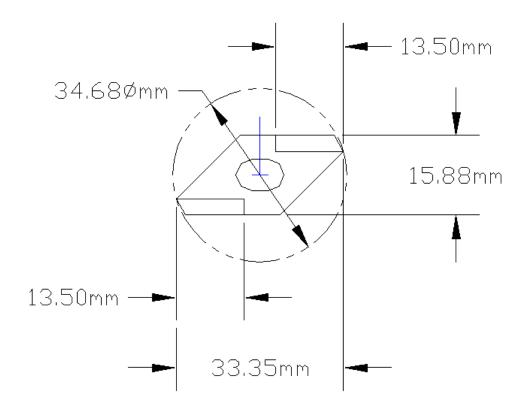
THE MAXIMUM TIP-SPEED BASED ON MAXIMUM SPEED OF THE CHOPPER BEING 10,000 R.P.M. = 10,000 R.P.M. / 60 SEC. = 166.66 R.P.S. X 0.109 = 18.16 M/SEC.
