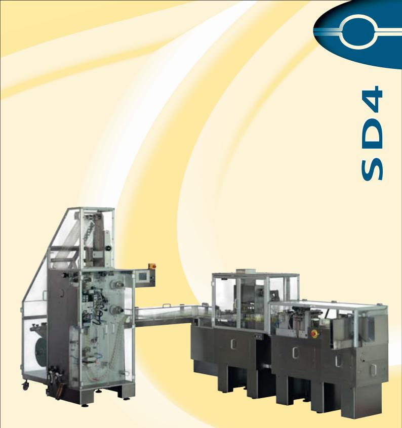
Automatic machine to produce unit-doses in plastic thermoformable materials for liquid and semiliquid products
