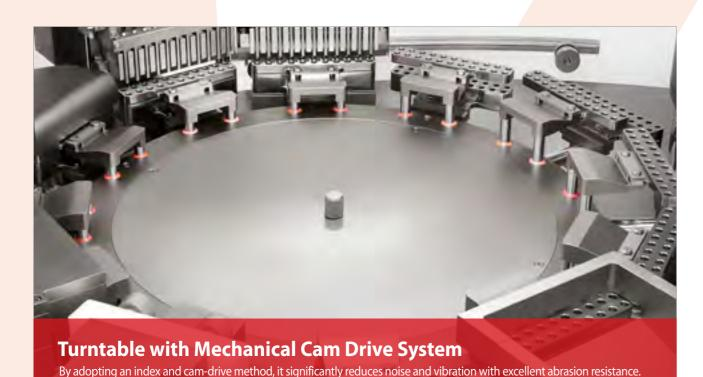
Through rotary motion delivered from a cam shaft, it transfers capsules to maintain each part's function.
