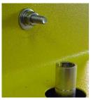
2.) Loosen the nut that holds the Pedestal Bolt in place, using a 10mm wrench, so that the Bolt can be moved out of the way. Next, move the Bolt as far in as possible, but do not let it fall into the machine.
